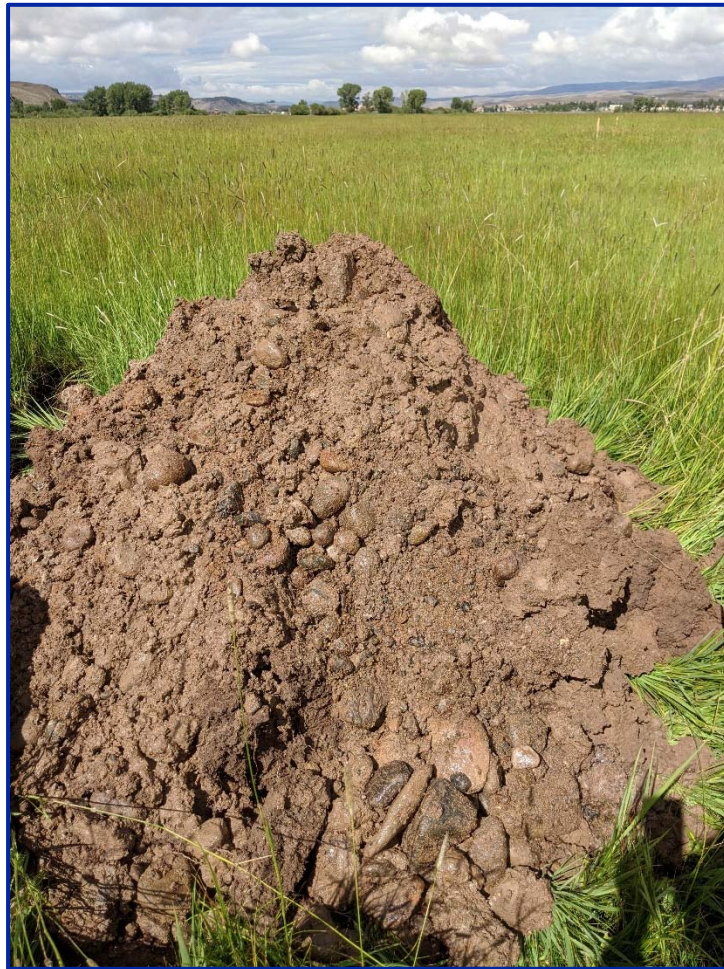
EXHIBIT 1. View of gravels encountered below the sandy clays in the exploratory pits.
